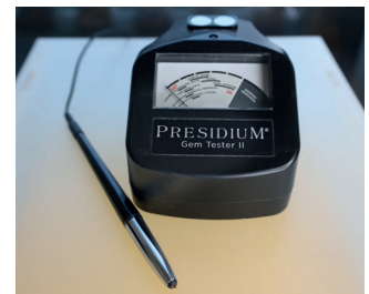
Lab-grown diamonds have nearly the same quality as mined diamonds. Testers read heat conductivity
