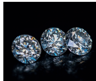
Lab-grown diamonds have nearly the same quality as mined diamonds. Testers read heat conductivity
